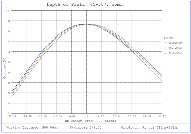
#85-367, 35mm, f/8 Ci Series Fixed Focal Length Lens, Depth of Field Plot, 300mm Working Distance, f8
