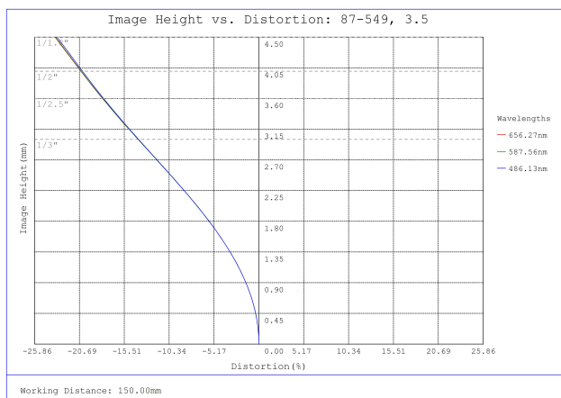
#87-549, 3.5mm, f/8 Ci Series Fixed Focal Length Lens, Distortion Plot
