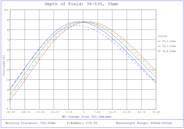
#36-530, 35mm f/8.0, HPr Series Fixed Focal Length Lens, Depth of Field Plot, 300mm Working Distance, f8
