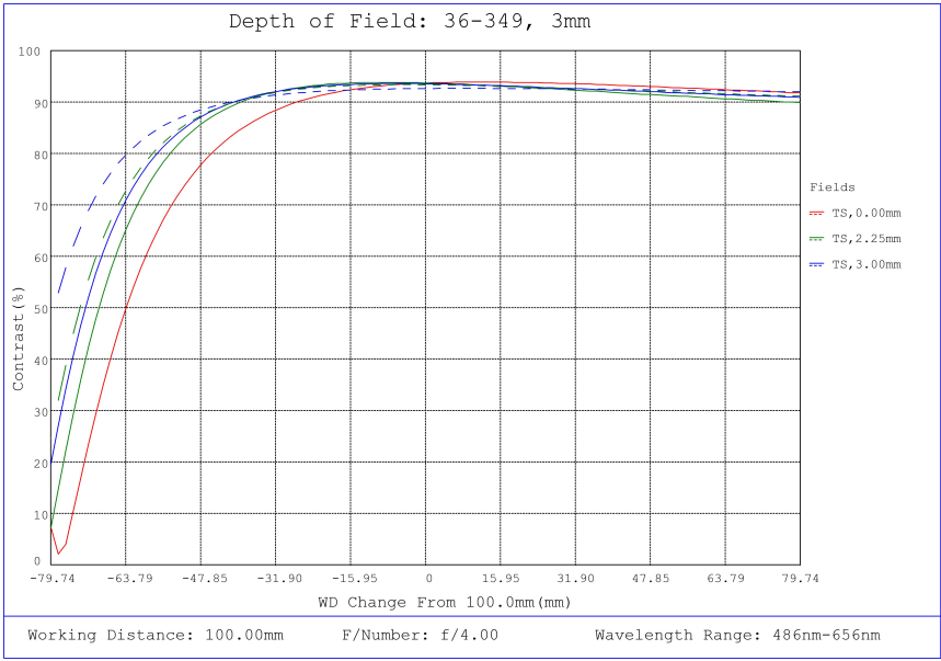
#36-349, 3mm FL f/4, Rugged Blue Series M12 Lens, Depth of Field Plot, 100mm Working Distance, f4
