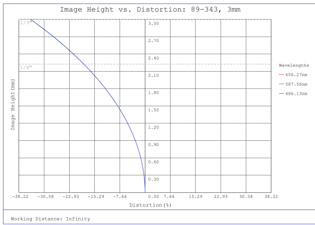
#89-343, 3mm FL f/8.0, Blue Series M12 Lens, Distortion Plot
