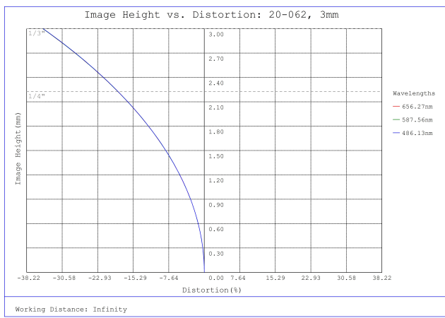
#20-062, 3mm FL f /8.0 IR-Cut Rugged Blue Series M12 Lens, Distortion Plot
