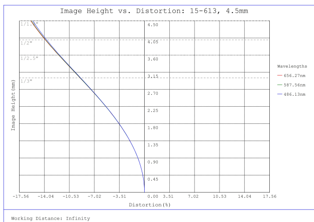
#15-613, 4.5mm f/2.0 Sealed Cw Series Fixed Focal Length Lens, Distortion Plot
