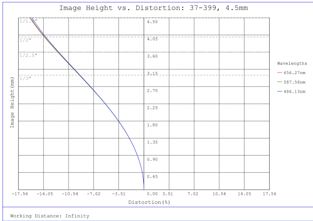
#37-399, 4.5mm, f/2.8 Cr Series Fixed Focal Length Lens, Distortion Plot
