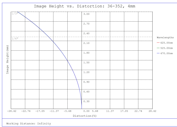
#36-352, 4mm FL f /2.5, Rugged Blue Series M12 Lens, Distortion Plot
