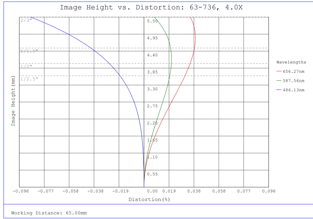
#63-736, 4X, 65mm WD CompactTL™ Telecentric Lens, Distortion Plot
