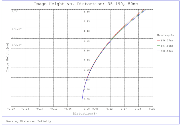
#35-190, 50mm, f/2.0 Cr Series Fixed Focal Length Lens, Distortion Plot
