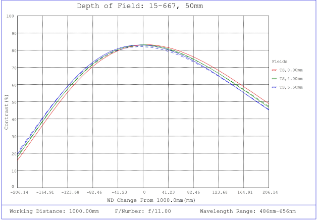
#15-667, 50mm, f/11 Sealed Cw Series Fixed Focal Length Lens, Depth of Field Plot, 1000mm Working Distance, f11
