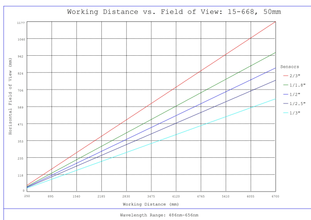
#15-668, 50mm, f/16 Sealed Cw Series Fixed Focal Length Lens, Working Distance versus Field of View Plot
