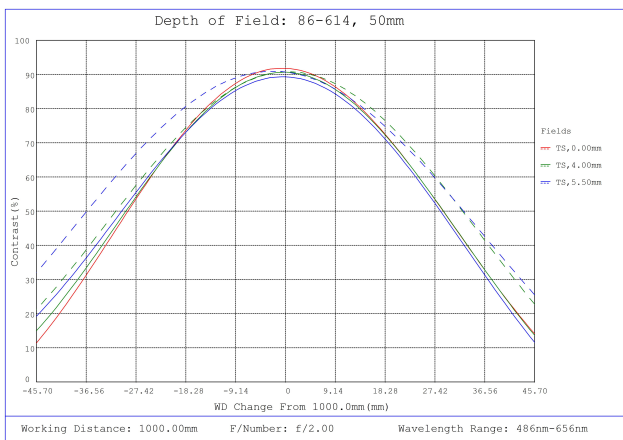
#86-614, 50mm, f/2.0 Ci Series Fixed Focal Length Lens, Depth of Field Plot, 1000mm Working Distance, f2
