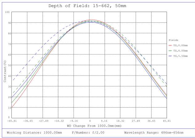
#15-662, 50mm, f/2.0 Sealed Cw Series Fixed Focal Length Lens, Depth of Field Plot, 1000mm Working Distance, f2
