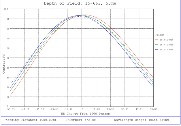
#15-663, 50mm, f/2.8 Sealed Cw Series Fixed Focal Length Lens, Depth of Field Plot, 1000mm Working Distance, f2.8
