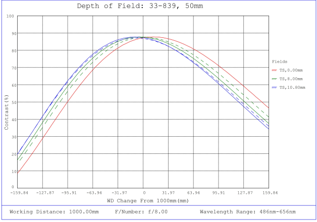
#33-839, 50mm f/8.0, HPi Series Fixed Focal Length Lens, Depth of Field Plot, 1000mm Working Distance, f8
