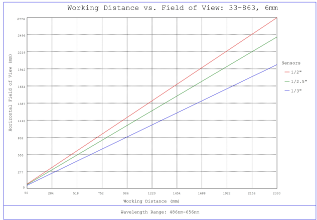
#33-863, 6mm, f/2.8 UCi Series Fixed Focal Length Lens, Working Distance versus Field of View Plot
