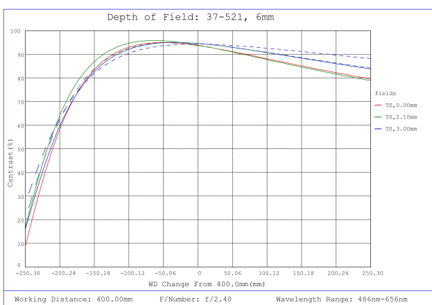
#37-521, 6mm FL, Liquid Lens M12 Lens, Modulated Transfer Function (MTF) Plot, 400mm Working Distance, f2.4
