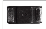
It's difficult to make an image of the electrode part using a Bar Light.
