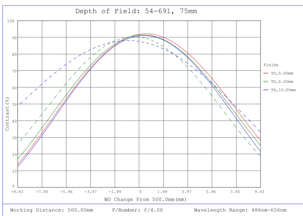
#54-691, 75mm DG Series Fixed Focal Length Lens, Depth of Field Plot, 500mm Working Distance, f4
