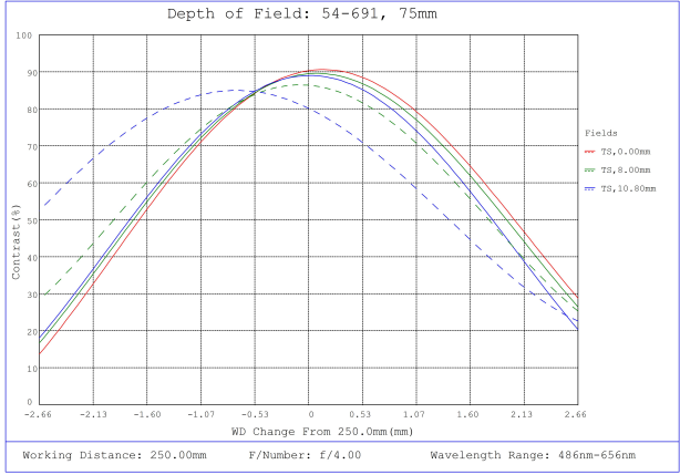
#54-691, 75mm DG Series Fixed Focal Length Lens, Depth of Field Plot, 250mm Working Distance, f4
