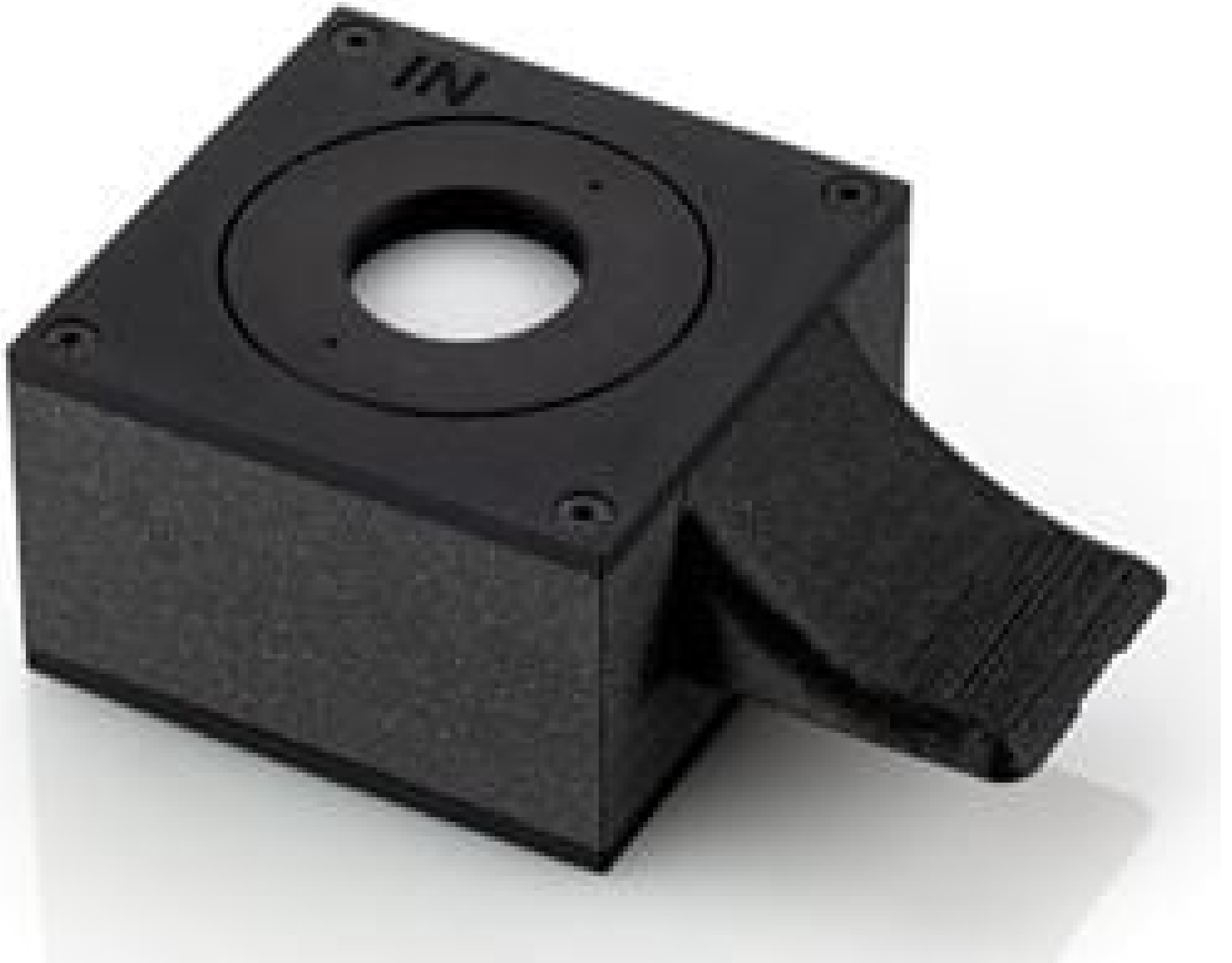
fNIRS Standard Phantom - IEC 80601-2-71
