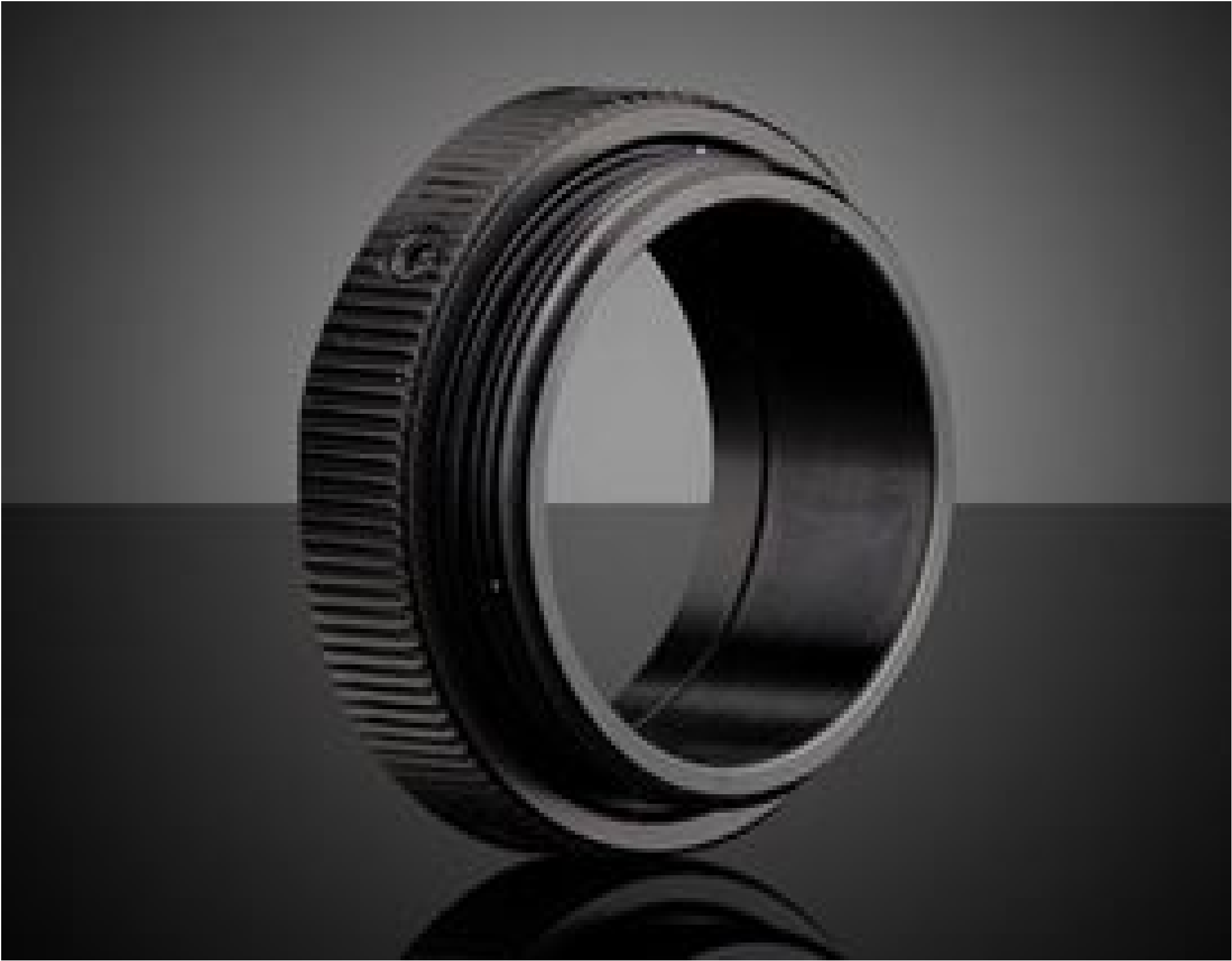
#66-381: M25.5 x 0.5 to C-Mount Rotating Male Adapter
