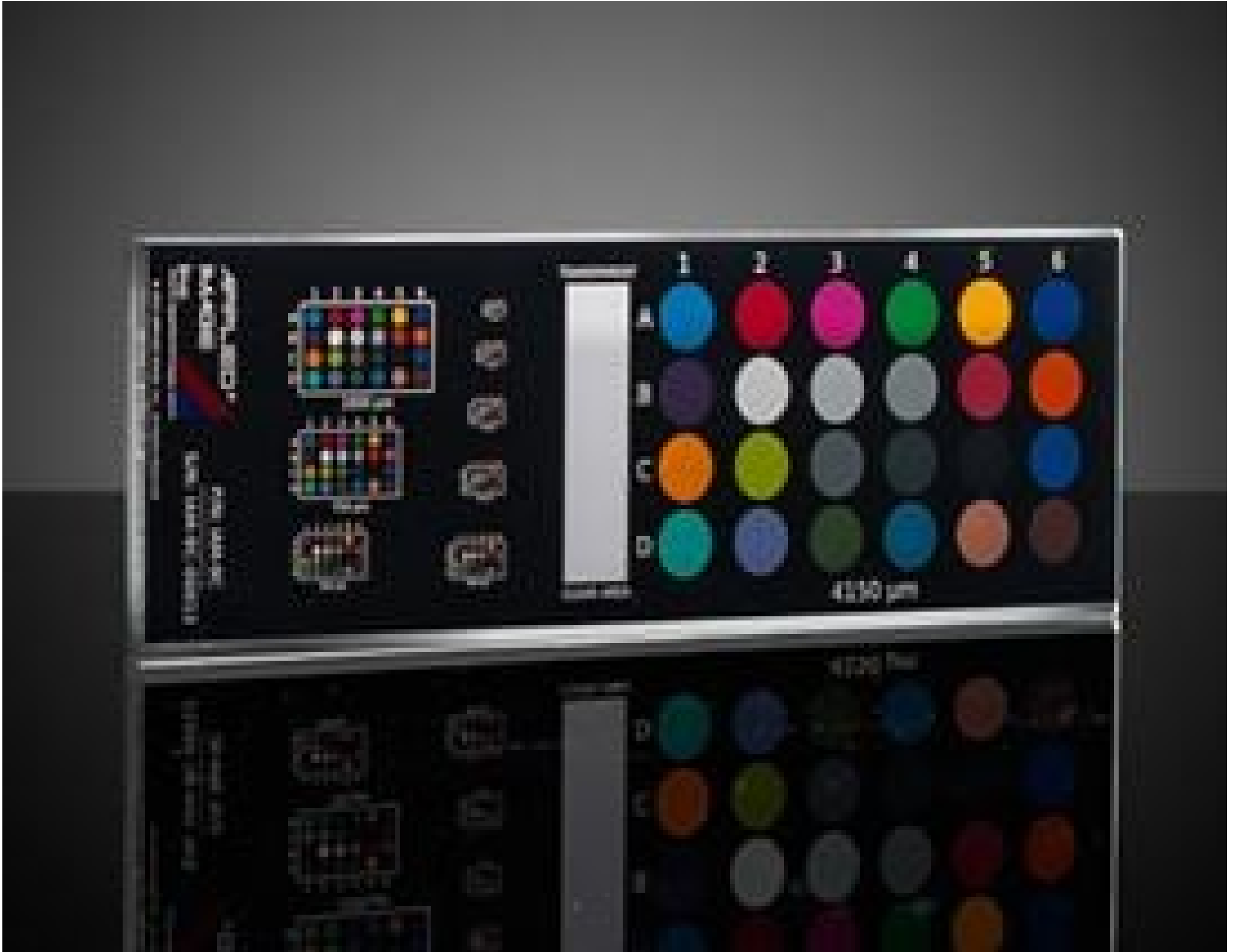
NIST Traceable Color Transmission Calibration Slides
